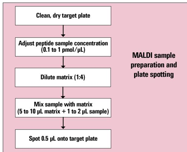
**Figure 2** Procedure for MALDI sample preparation
