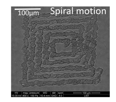
→ Laser ablation following a Spiral motion in HCCA matrix inspected by Scanning Electron Microscopy
