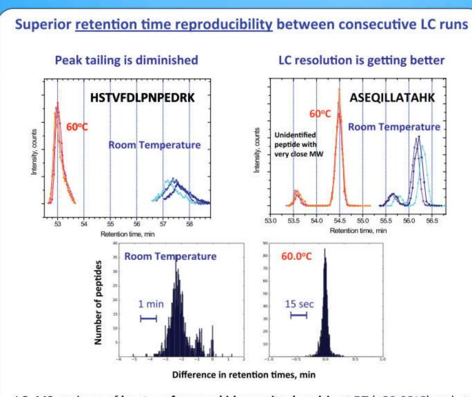
LC- MS analyses of lysates of mouse kidney mitochondria at RT (~20-22°C) and at 60.0°C. Significant improvement in chromatographic reproducibility, resolution, decrease in peak tailing, increase in peak heights.
