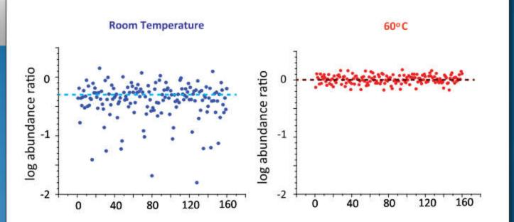
Normalized areas of 160 LC peaks from the LC-MS analysis of a 10-protein digest. LC separations were performed using a 40-min long gradient at room temperature and at 60°C in triplicates.
