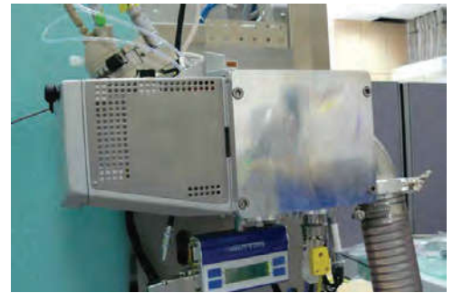
Ion funnel interface coupled to a Thermo Orbitrap
