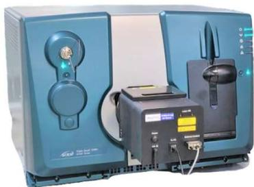
Figure 1. AP/MALDI coupled with SCIEX QTRAP 6500plus system
