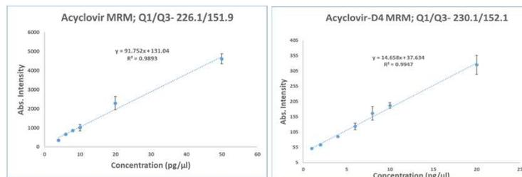
Figure 3. Calibration curves for MRM transition of acyclovir and acyclovir-D4 spotted on stainless still MALDI target plate
