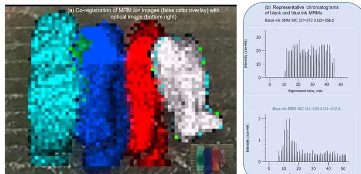
Figure 5. AP/MALDI MRM MSI reconstructed ion images of permanent marker inks co-registered with optical image and (b) selected ion chromatograms of black and blue permanent marker inks. Image generated using Mozaic software from Spectroswiss Sarl.
