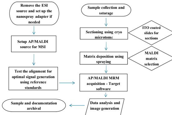
Figure 2. Workflow for mass spectrometry imaging using AP/MALDI ionization source
