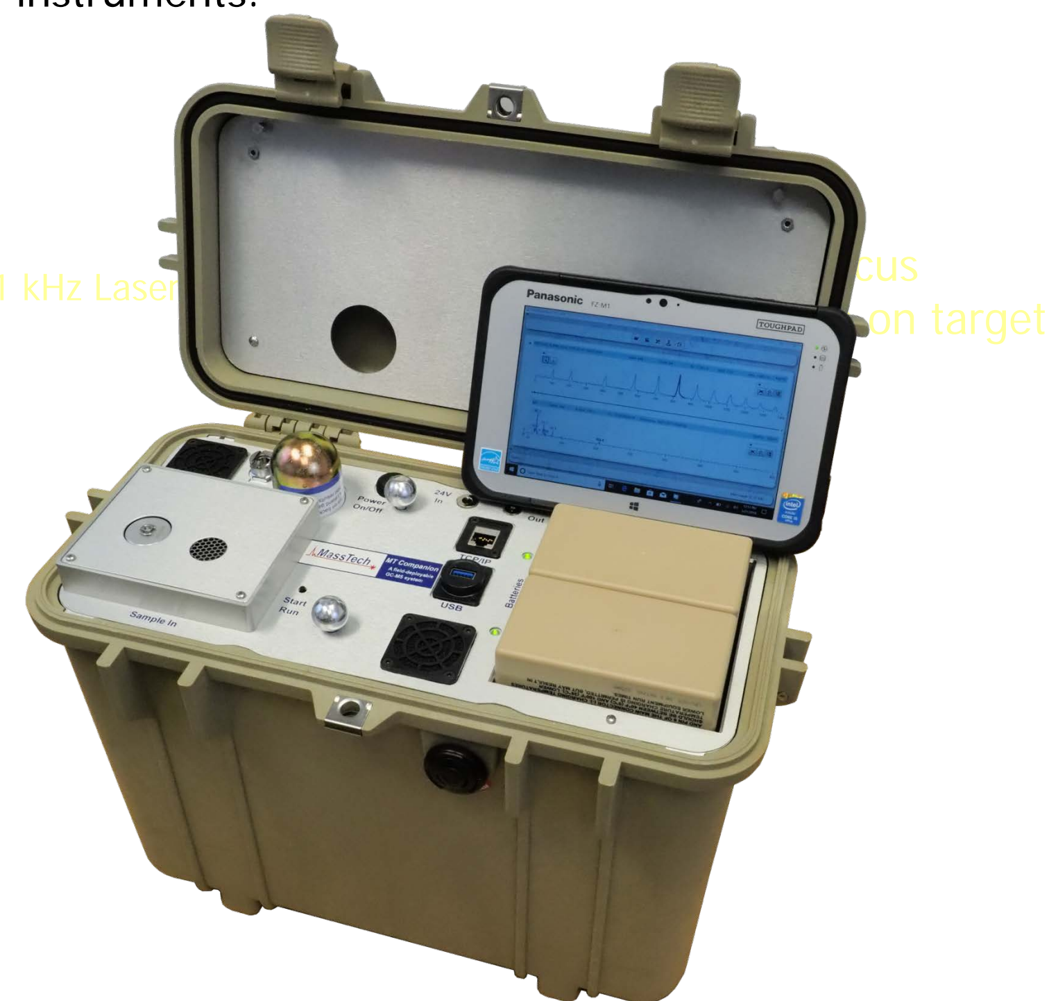
A general view of \mu GC/MS instrument in a waterproof enclosure of 16.9 x 9.6 x 13.4" dimensions
