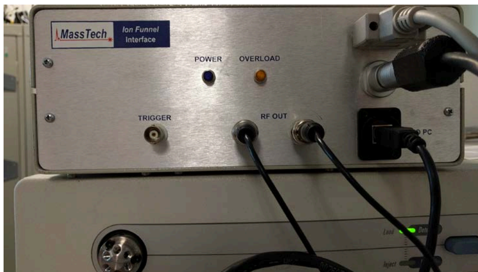
Figure 5.8. Connecting cables to DC/RF box
