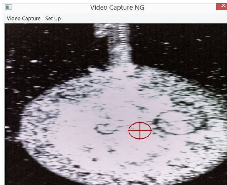
Figure 7.4 Positioning the Red (Laser) Cross Hairs
