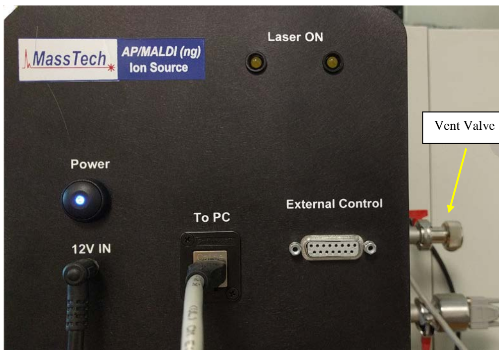
Figure 5.2. Control unit for the Thermo Mass Spectrometer with inserted Ethernet cable and power cord from 12 V power supply
