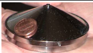
Fig 5.7. The Ion Sweep Cone Must be Removed Prior to Source Installation
