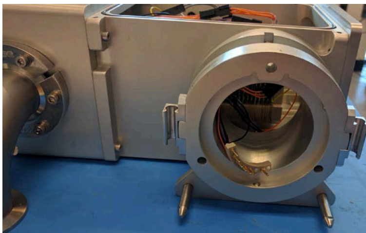
Figure 5.2. A view of the two-stage Ion Funnel. The heated capillary cone is not installed. In the heated cone mounting hole, one can see the wired PEEK segment connector with 7 pins. The pins should be inserted into opposite bronze receptacles in the inlet capillary cone taken from Thermo MS.
