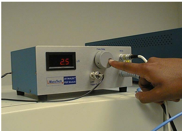
Figure 14. Pulse Delay adjustment knob
