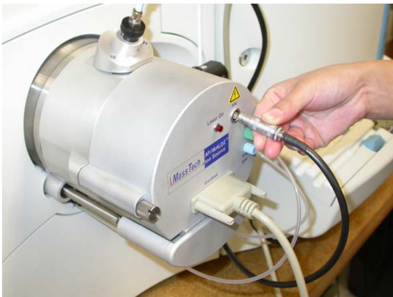
Figure 9. Connect the HV Out cable from the PDF Module into the AP/MALDI ion source.
