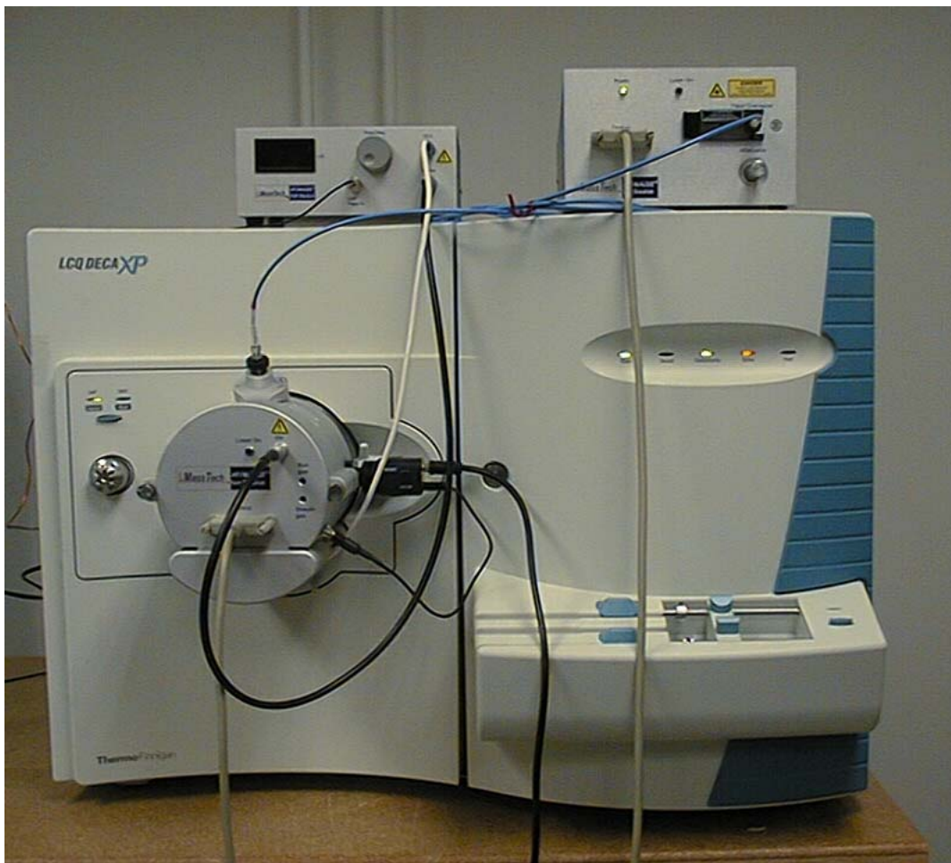
Figure 13. PDF Module fully connected to an AP/MALDI ion source
