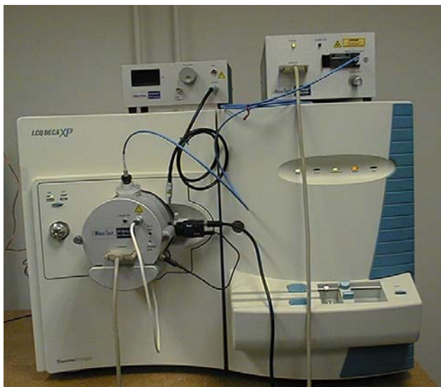
Figure 5. PDF Module located in close proximity to the AP/MALDI ion source and LCQ HV Cable.
