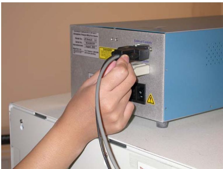
Figure 10. Connect the External Controls Cable to the External Controls output on the rear panel of the AP/MALDI Control Unit.
