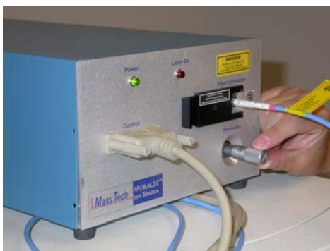
Figure 18. Increase laser energy on the AP/MALDI Control Unit.
