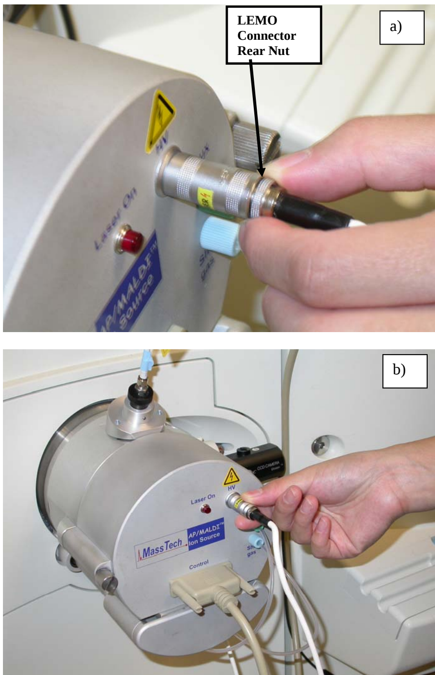
Figure 7a, 7b. Disconnect the LCQ HV Cable from the AP/MALDI ion source by a) loosening the rear nut on the LEMO connector and b) pulling the connector off.
