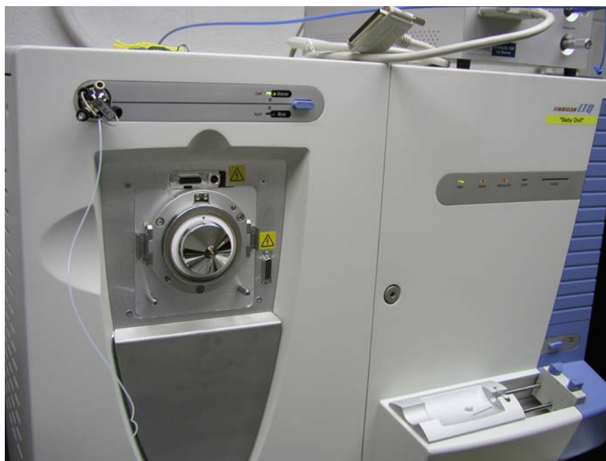
Fig 5-8 LTQ without any ion source attached, and Ion Sweep Cone Removed.
