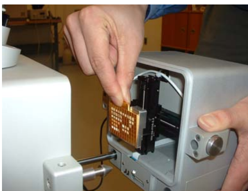
Fig. 6-3 Handling the Target Plate with the prepared sample spots into the Target Plate Holder. The Plate is held in place by a magnet. Caution – the Target Plate may be hot when unloading.
