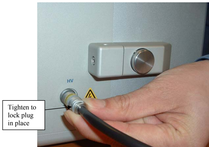
Fig. 5-17. HV Cable Connection. Tightening the knurled back end of the HV plug locks the cable in place.
