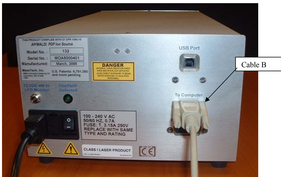
Fig. 5-10 The black power cord and Cable B (RS232 Serial Cable option shown here) connected to the back of the Control Unit. No adjustment is necessary for ~110/~127/~220/~240V AC!
