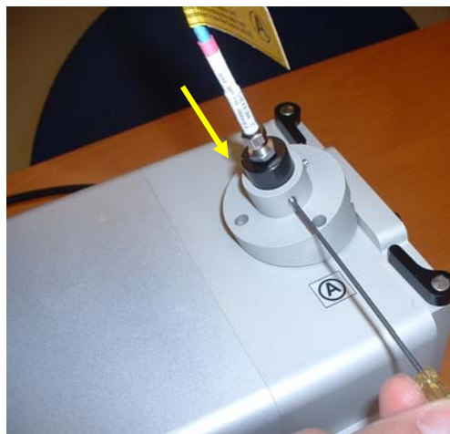
Fig. 7-20. Adjustment of the focusing tube on the AP/MALDI ion source to defocus the laser beam.
