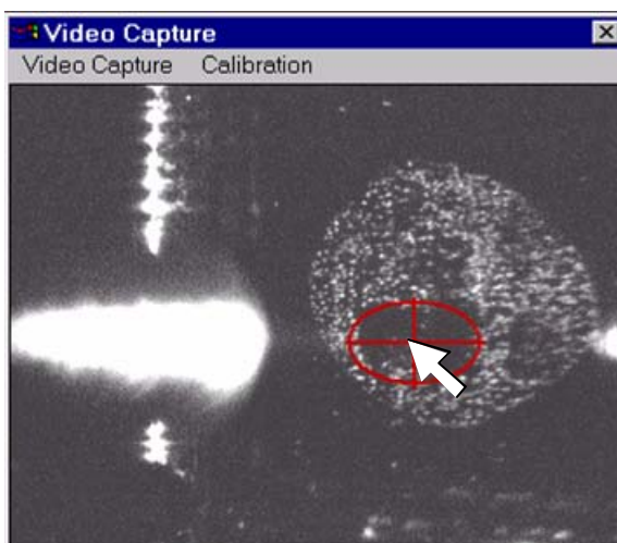
Fig. 7-5 Resizing of the Red (Laser) Target by placing the mouse at the center of the Red Cross Hairs, pressing Shift and dragging the mouse to resize the area.
