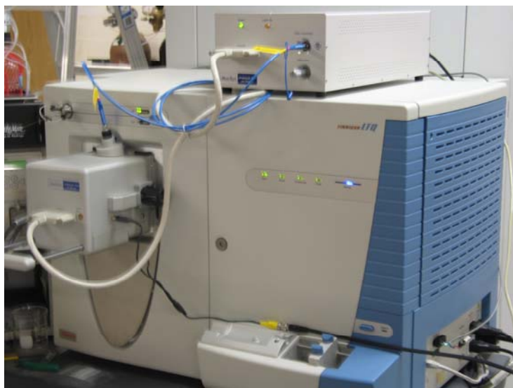
Fig. 5-18 Completed source installation. (Note: In this picture, camera power cable is plugged into Target Side Flange, although it is normally plugged into Instrument Side Flange)
