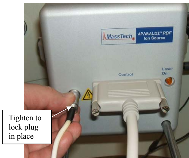
Fig. 5-20. HV Cable Connection. Tightening the knurled back end of the HV plug locks the cable in place.
