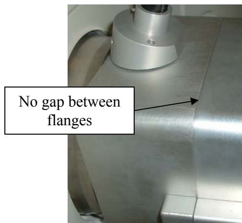
Fig. 6-4 The Source into the close position after target (sample) plate is loaded. Notice that there is no gap between the two halves of the ion source.
