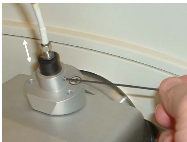
Fig. 5-24. Laser Focused by loosening side set screw, adjusting focusing optic up/down, and then retightening set screw.
