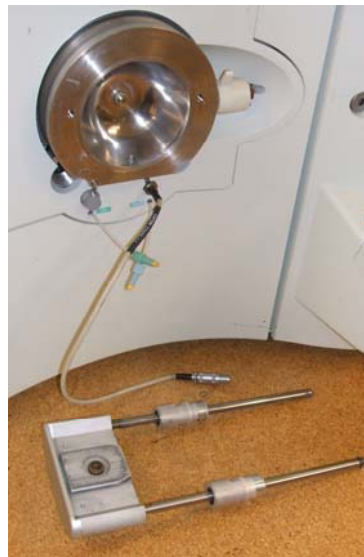
Fig 5-10 LCQ instrument ready for AP/MALDI source installation.
