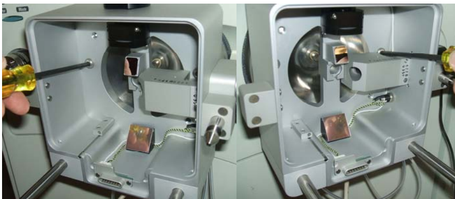
Fig 5-11 Screwing AP/MALDI-PDF source onto the LCQ inlet flange.
