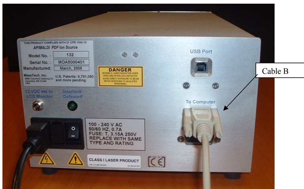
Fig. 5-13 The black power cord and USB Cable B connected to the back of the Control Unit. No adjustment is necessary for ~110/~127/~220/ ~240V AC!
