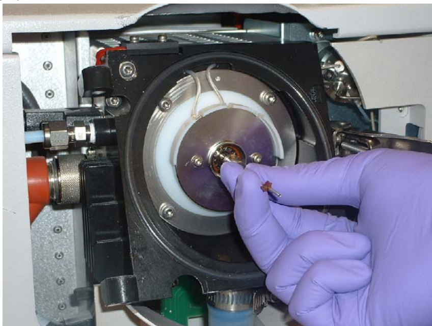
Fig 5-10 Installing the Capillary extension to the LC/MSD.
