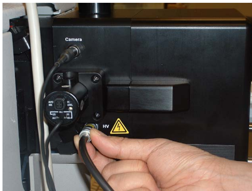
Fig. 5-22. HV Cable Connection.
