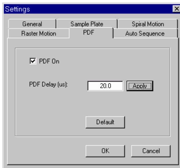
Figure 7-18. Pulse Delay adjustment
