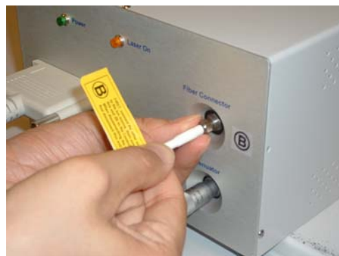
Fig. 5-21 Connecting the fiber to the Control Unit (B to B)
