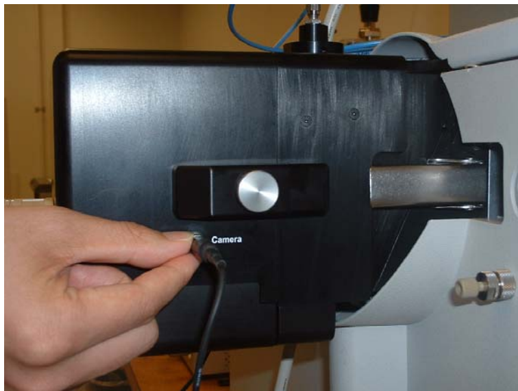
Fig. 5-24 CCD camera alternative power cable connection for adjustments
