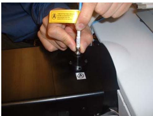
Fig. 5-20 Connecting fiber to Source (A to A)
