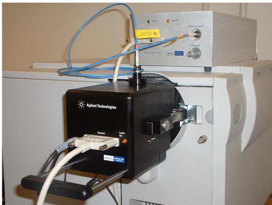
Fig. 6-4 Source "Clicked" into the close position after target (sample) plate is loaded.
