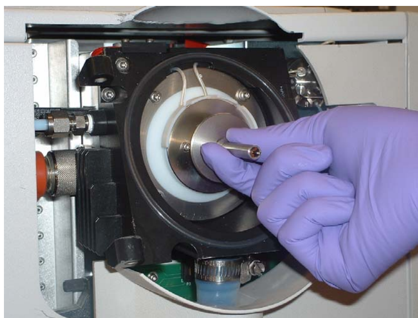
Fig 5-11 Installing the Heating Sleeve over the Capillary extension
