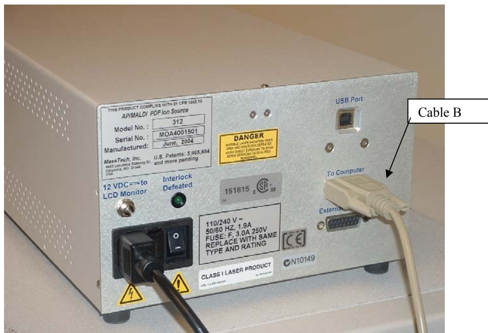
Fig. 5-16 The black power cord and Cable B connected to the back of the Control Unit. No adjustment is necessary for ~110/~127/~220/~240V AC!
