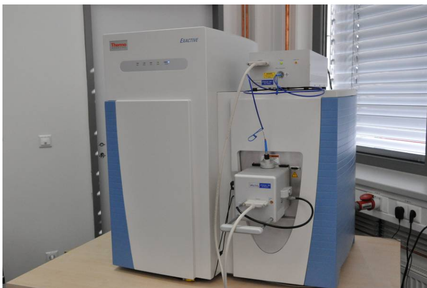
Fig. 5-18 Completed source installation.
