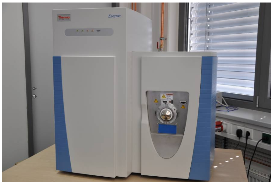
Fig 5-8 Exactive without any ion source attached, and Ion Sweep Cone Removed.
