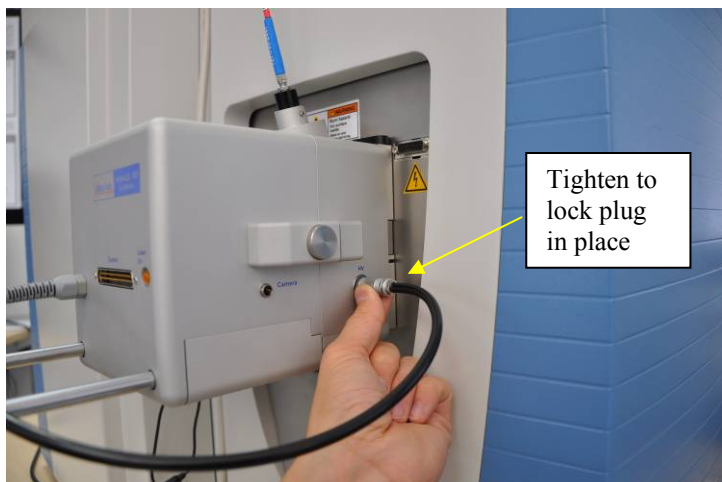
Fig. 5-17. HV Cable Connection. Tightening the knurled back end of the HV plug locks the cable in place.
