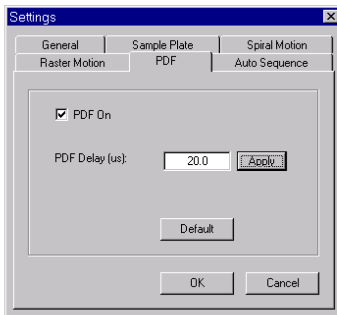
Figure 7-21. Pulse Delay adjustment
