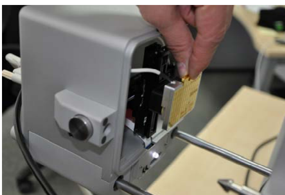
Fig. 6-3 Handling the Target Plate with the prepared sample spots into the Target Plate Holder. The Plate is held in place by a magnet.
