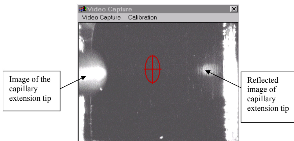
Fig. 8-2 Blank sample spot on the Video Capture screen
