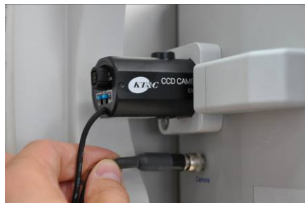
Fig. 5-19 CCD camera alternative power cable connection for adjustments
