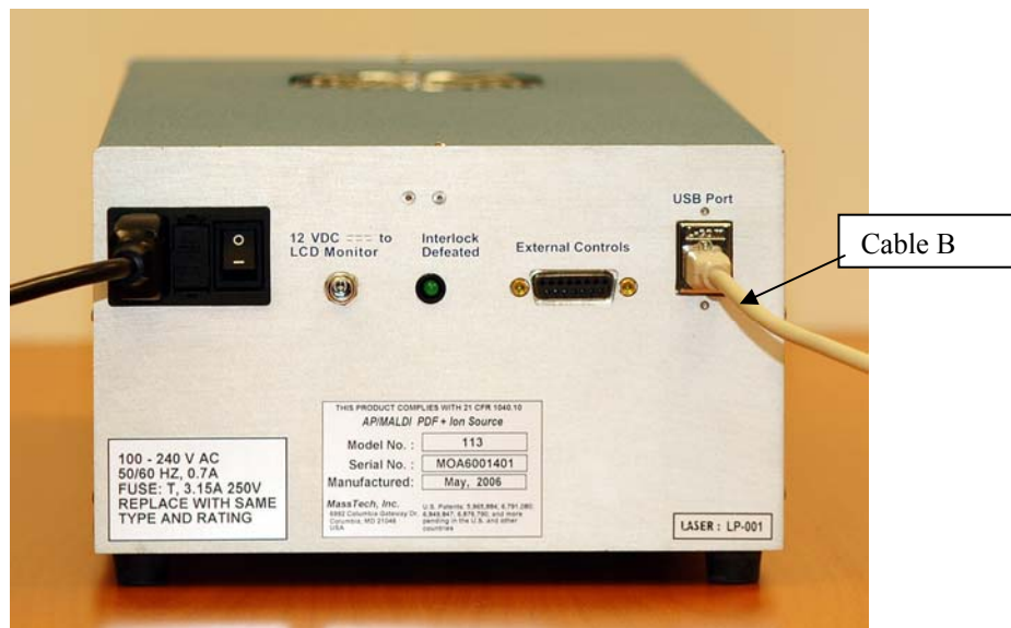
Fig. 5-10 The black power cord and USB Cable B connected to the back of the Control Unit. No adjustment is necessary for ~110/~127/~220/~240V AC!
