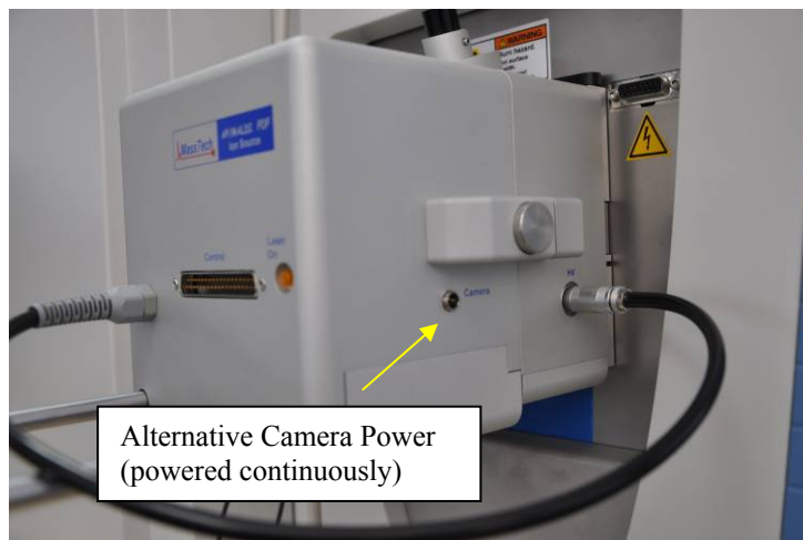
Fig. 5-13 Normal connection for Camera power cable. Alternative power port is to maintain imaging while source is open, and is used for testing/tuning purposes only.
