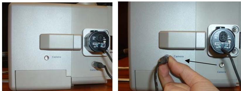
Fig. 5-19 CCD camera alternative power cable connection for adjustments
