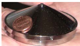
Fig 5-9b Ion Sweep Cone removed prior to source installation. CAUTION: Ion Sweep Cone may be hot!
