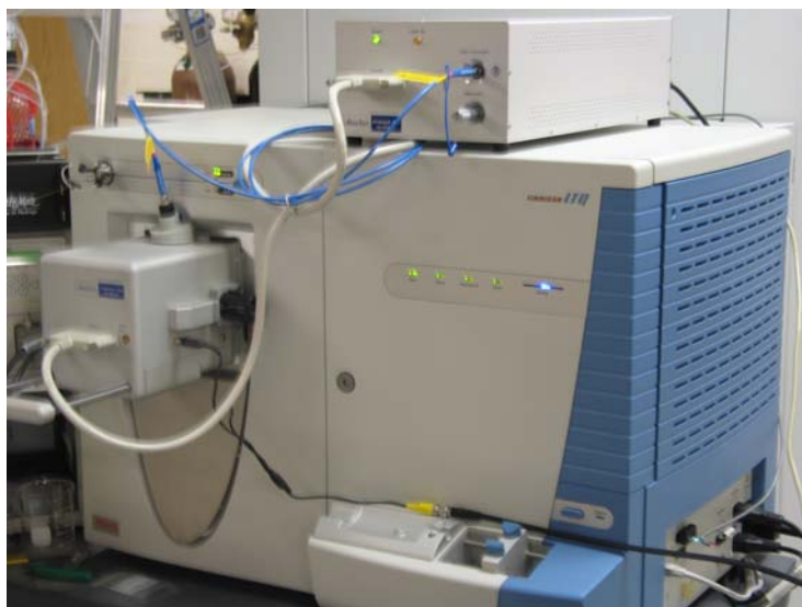
Fig. 5-18 Completed source installation.
