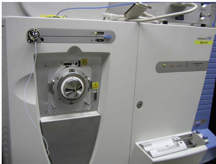
Fig 5-8 LTQ without any ion source attached, and Ion Sweep Cone Removed.
