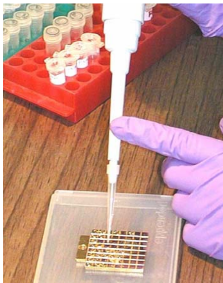
Fig. 6-1 Spotting of several standard samples on a target (sample) plate for testing by AP/MALDI. The sample preparation procedure is basically the same as for original MALDI experiments.
