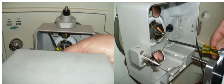
Fig 5-10 Screwing AP/MALDI source onto the LCQ inlet flange.
