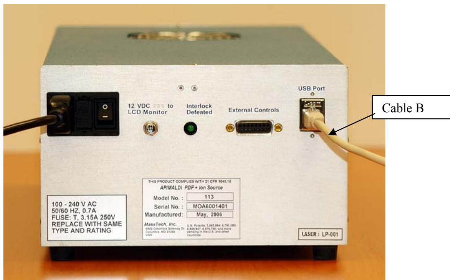
Fig. 5-11 The black power cord and USB Cable B connected to the back of the Control Unit. No adjustment is necessary for ~110/~127/ ~220/ ~240V AC!
