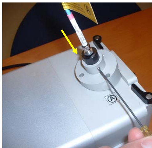
Fig. 7-23. Adjustment of the focusing tube on the AP/MALDI ion source to defocus the laser beam.
