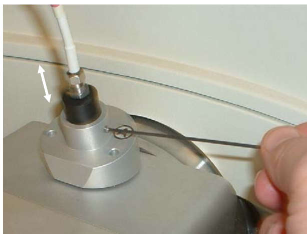
Fig. 5-22. Laser Focused by loosening side set screw, adjusting focusing optic up/down, and then retightening set screw.
