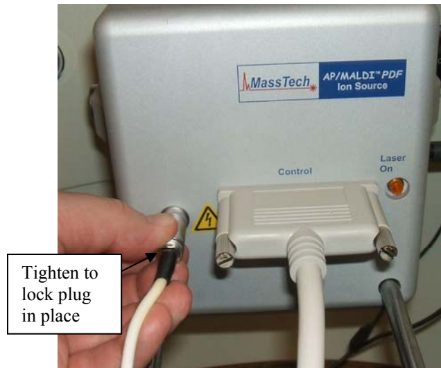
Fig. 5-18. HV Cable Connection. Tightening the knurled back end of the HV plug locks the cable in place.
