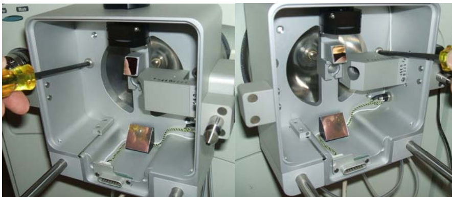
Fig 5-11 Screwing AP/MALDI PDF source onto the LCQ inlet flange.
