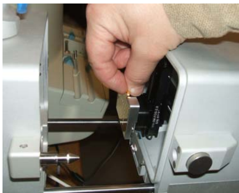
Fig. 6-3 Handling the Target Plate with the prepared sample spots into the Target Plate Holder. The Plate is held in place by a magnet.
