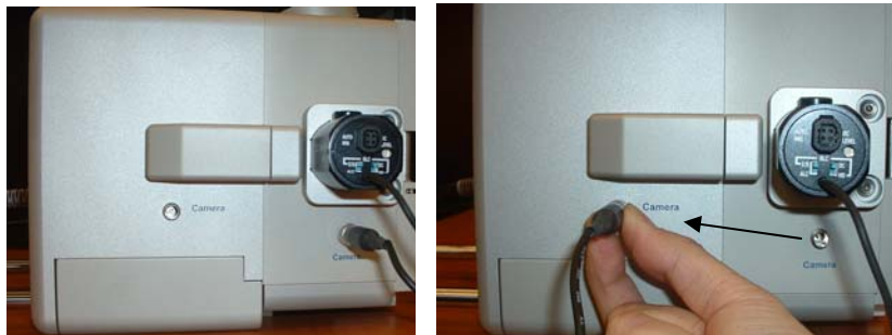
Fig. 5-21 CCD camera alternative power cable connection for adjustments
