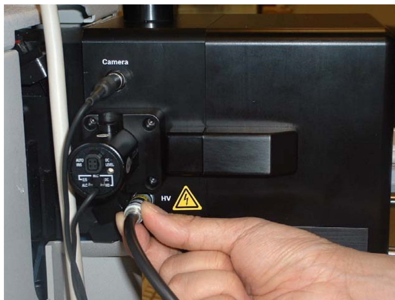
Fig. 5-22. HV Cable Connection.
