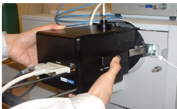
Fig. 6-2 Opening the source by pressing the round silver Locking button and pulling the Target Side of the source away from the instrument.
