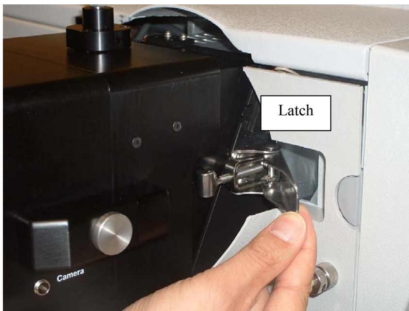
Fig 5-15 Securing both halves of the source and anchoring with the latch on the LC/MSD.
