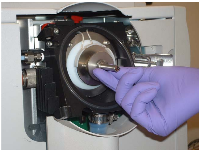
Fig 5-12 Placing the Wave disk spring over the Heating Sleeve
