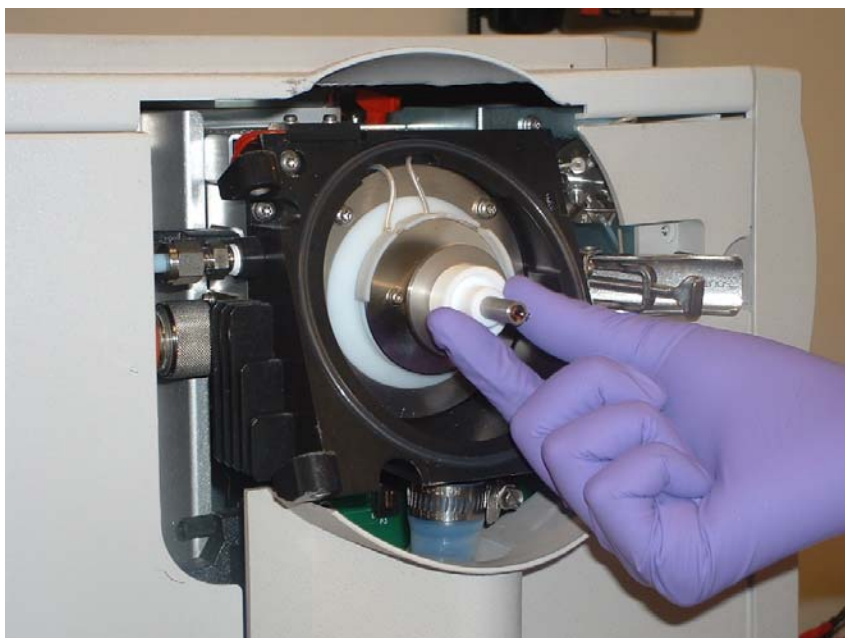
Fig 5-13 Finishing the Capillary Extension Assembly by adding the Teflon Centering Bushing
