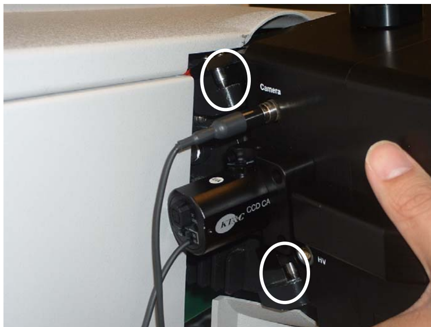
Fig 5-14 Hinging the source into place on the LC/MSD
