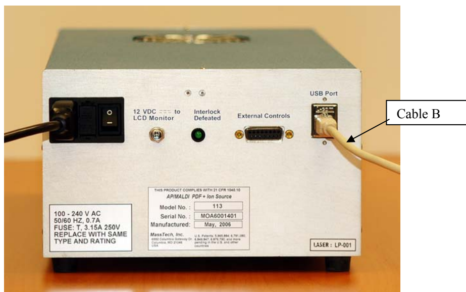
Fig. 5-16 The black power cord and Cable B connected to the back of the Control Unit. No adjustment is necessary for ~110/~127/~220/~240V AC!
