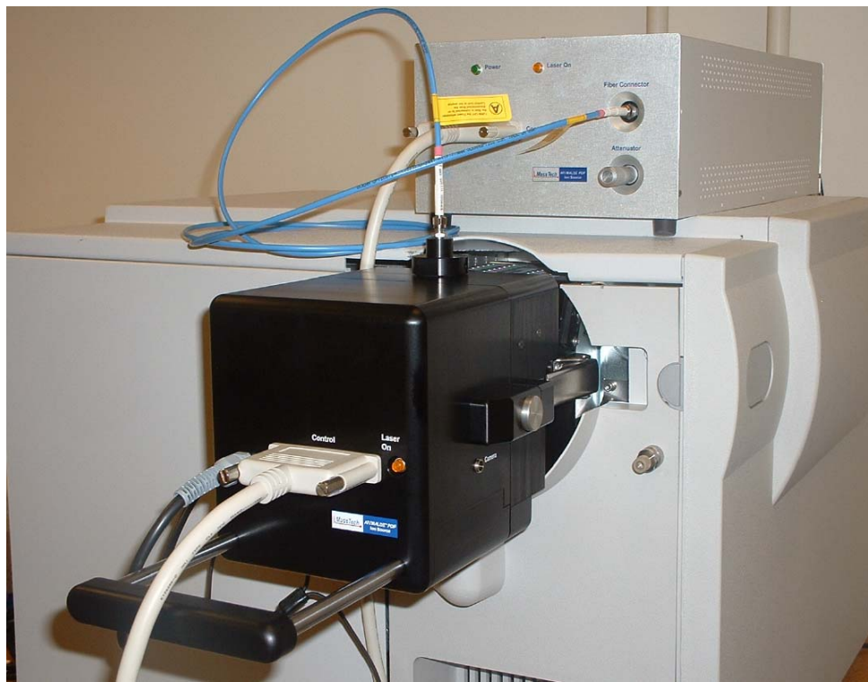
Fig. 6-4 Source "Clicked" into the close position after target (sample) plate is loaded.
