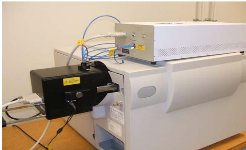
Fig. 5-23 Completed source installation
