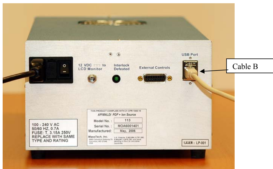
Fig. 5-17 The black power cord and Cable B connected to the back of the Control Unit. No adjustment is necessary for ~110/~127/~220/~240V AC!
