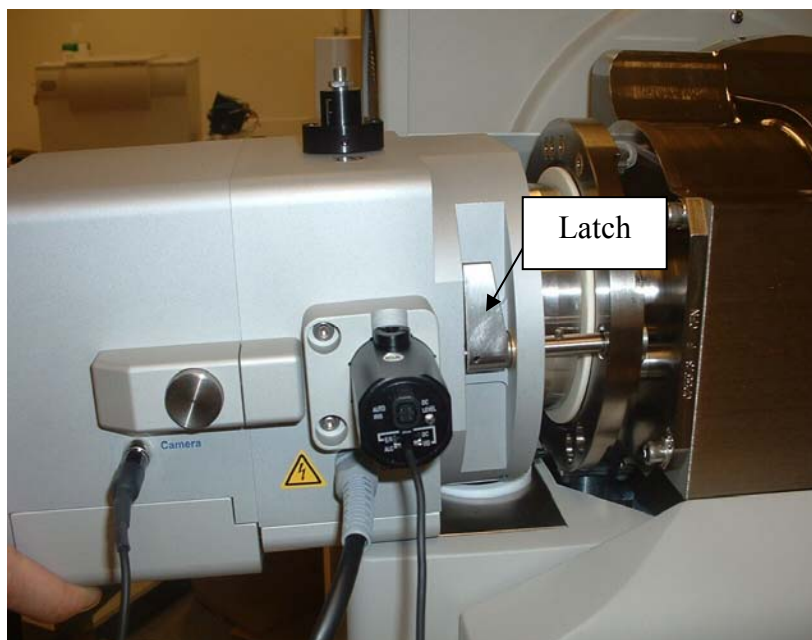
Fig 5-15 Mounting of AP/MALDI source to the Q-trap.
