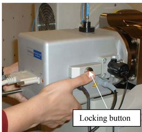
Fig. 6-2 Opening the source by pressing the round silver Locking button and pulling the Target Side of the source away from the instrument.
