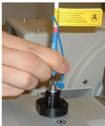
Fig. 5-21 Connecting fiber to Source (A to A)
