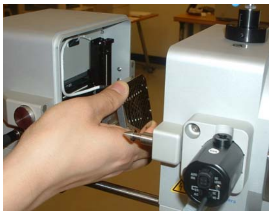
Fig. 6-3 Handling the Target Plate with the prepared sample spots into the Target Plate Holder. The Plate is held in place by a magnet. Caution – the Target Plate may be hot when unloading.
