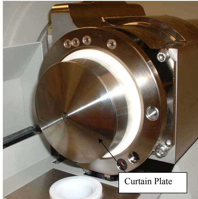
Fig 5-8 The inlet flange of Q-trap instrument configured for Nanospray (Curtain Plate On).
