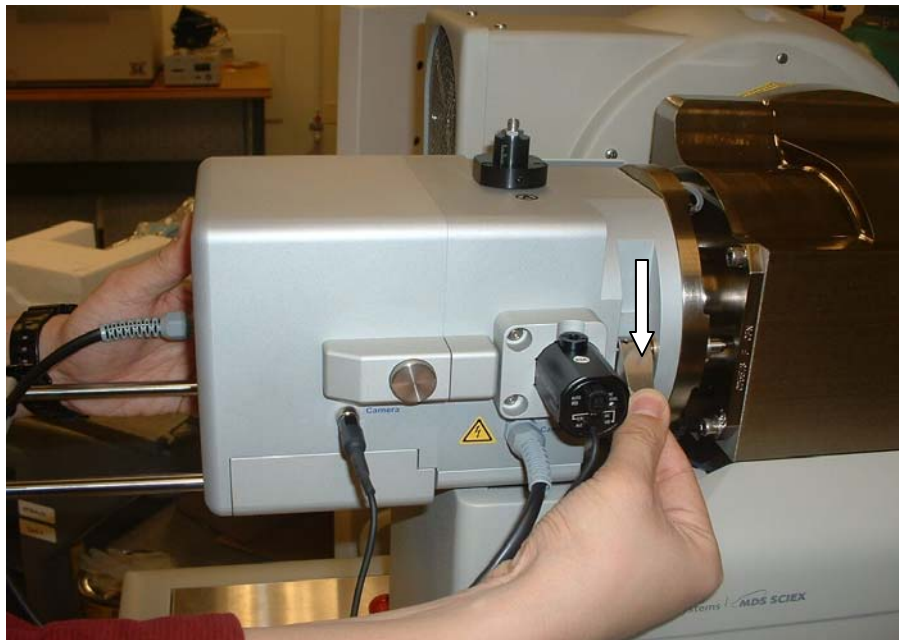
Fig 5-16 Latching of AP/MALDI source installed to the Q-trap.
