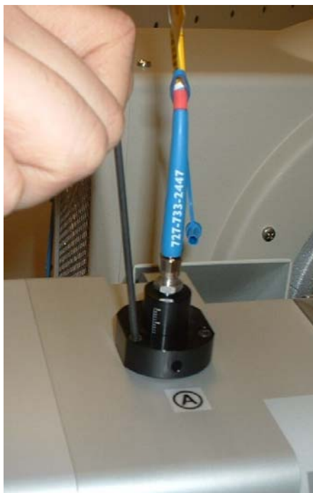
Fig. 5-26. Laser Positioned by adjusting three top screws.
