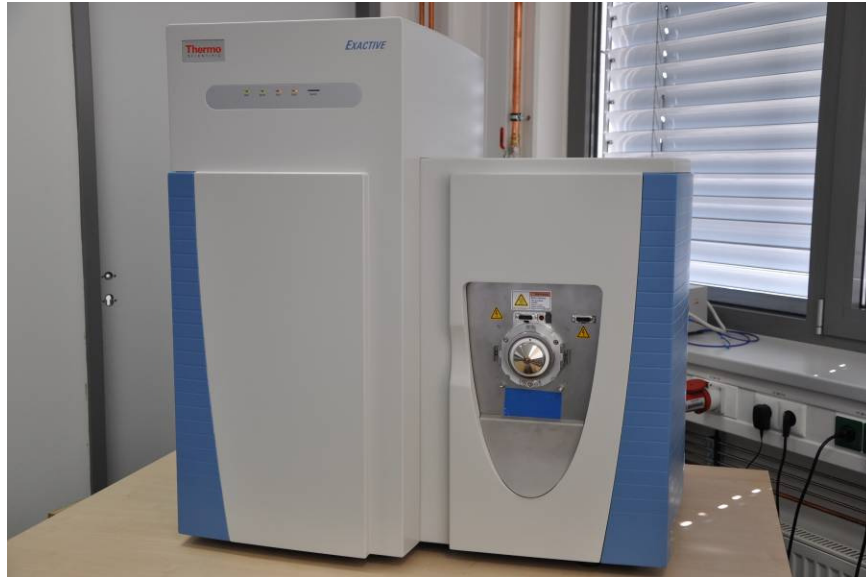
Figure 5.8 The Mass Spectrometer without the Ion Source and Ion Sweep Cone Attachment
