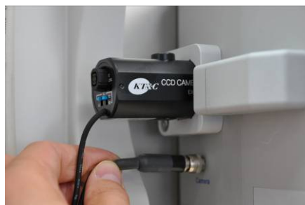
Figure 5.19 The Alternative Power Cable Connection for the CCD Camera
