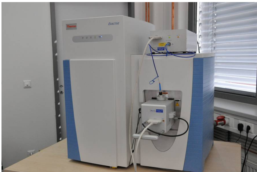
Figure 5.18 Completed Source Installation (Note: In this picture, camera power cable is plugged into Target Side Flange, although it is normally plugged into Instrument Side Flange)
