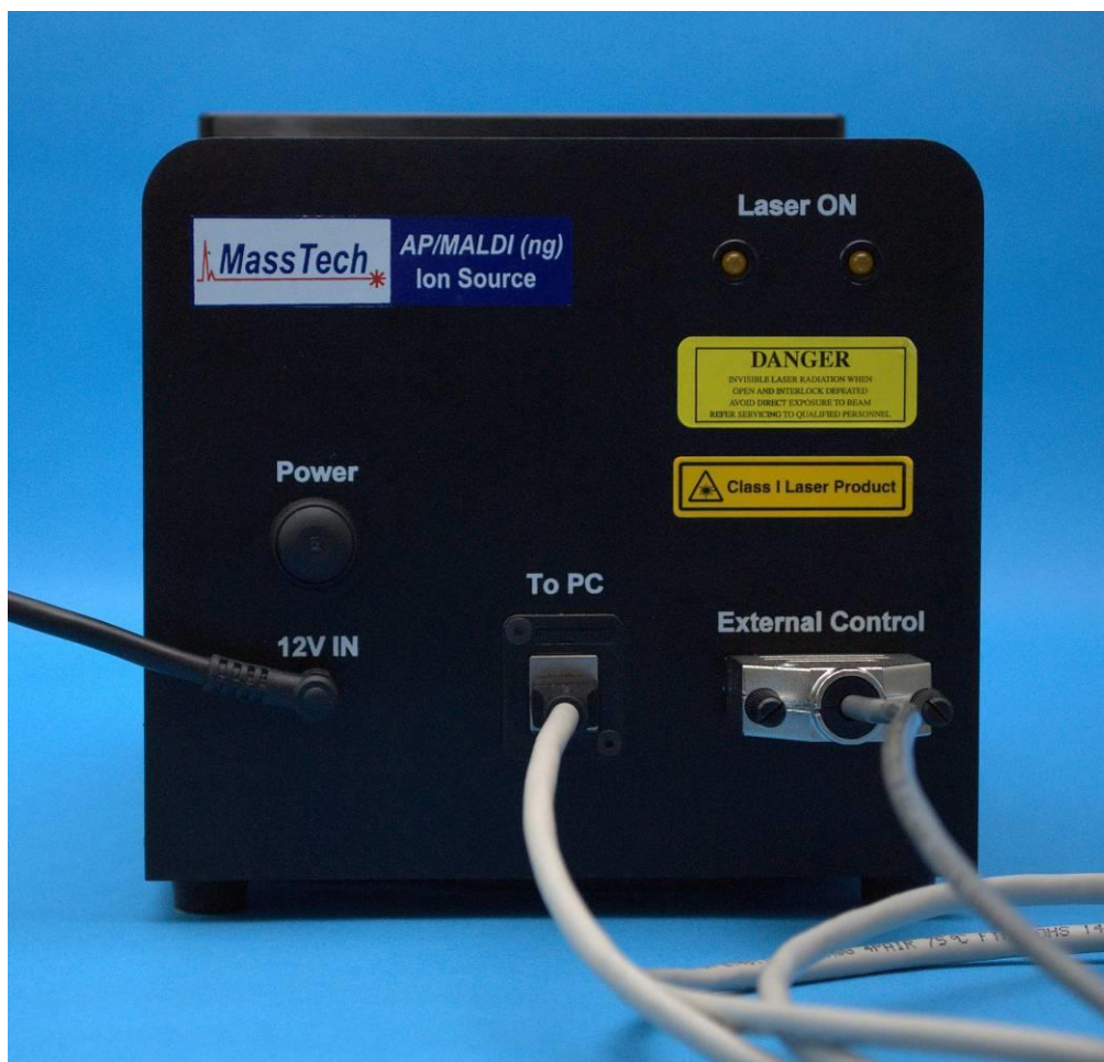
Fig 5.12 AP/MALDI (ng) Source with Power, PC, and External Control Cables
