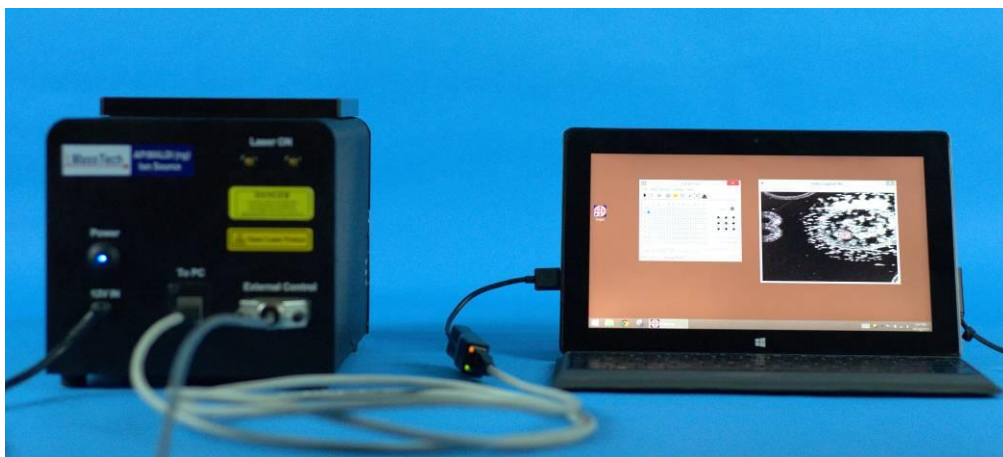
Fig 5.13 AP/MALDI (ng) Source with Power, PC, and External Control Cables
