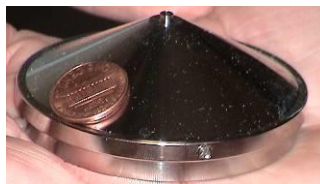
Fig 5.8c The Ion Sweep Cone Removed Prior to Source Installation
