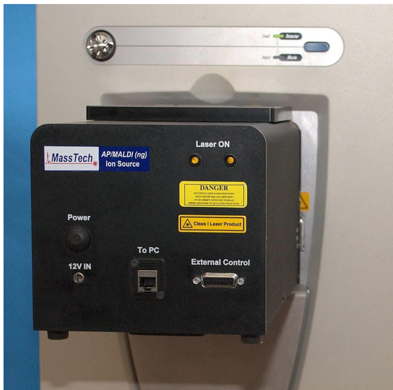
Figure 8.2 AP/MALDI (ng) installed on LCQ instrument
