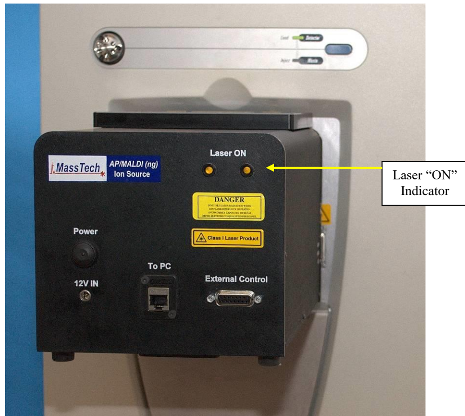
Figure 5.2 Ion Source for the Thermo Mass Spectrometer
