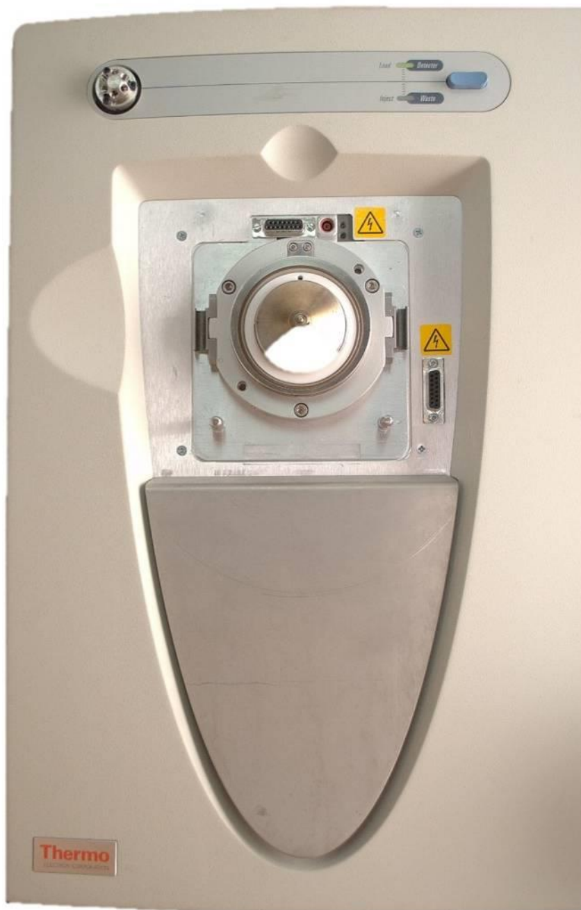
Figure 5.7 The Mass Spectrometer without the Ion Source and Ion Sweep Cone Attachment
