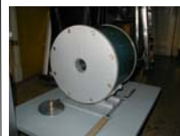
Figure 9. 2.1 T permanent with 5 cm bore and 75 kg weight. Field homogeneity (no shimming) is 500 ppm.
