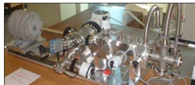
Figure 4. 0.97T permanent magnet FTICR instrument with atmospheric pressure ionization source: SolidWorks model (top) and photo of the built instrument (bottom).
